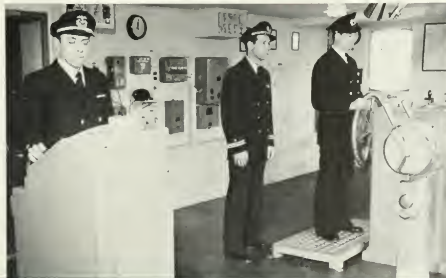
SCENE ON BRIDGE OF THE INDEPENDENCE SHOWING, AT LEFT, THE RCA RADAR UNIT WHICH CAN DETECT OBJECTS WITHIN A 40-MILE RANGE.
