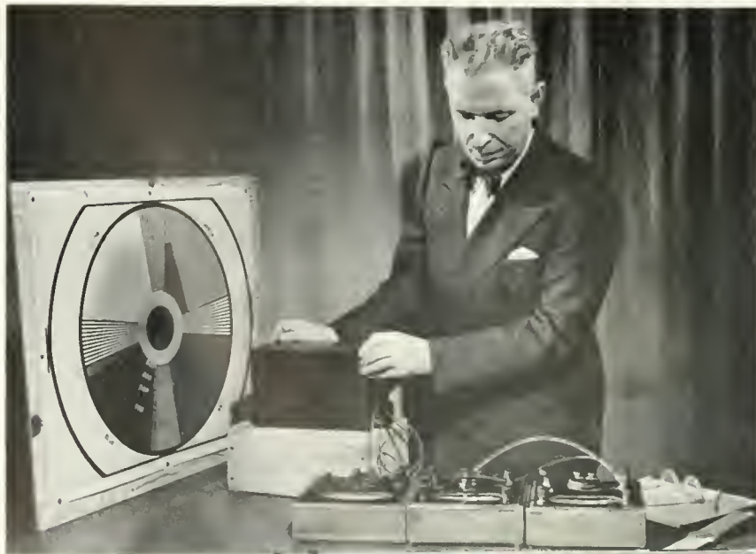
GEORGE C. SZIKLAI, OF RCA LABORATORIES, DEMONSTRATES THE TRISTIMULUS PHOTOMETER, WHICH PERMITS RAPID ANALYSIS OF COLORS.
